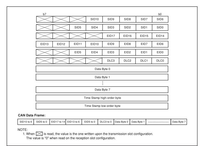
Figure 18.2 Bit Mapping in Byte Access
